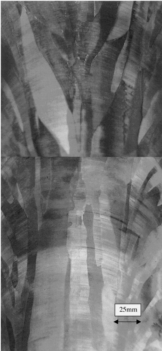
Fig. 3. A macrograph of a tantalum ingot.
